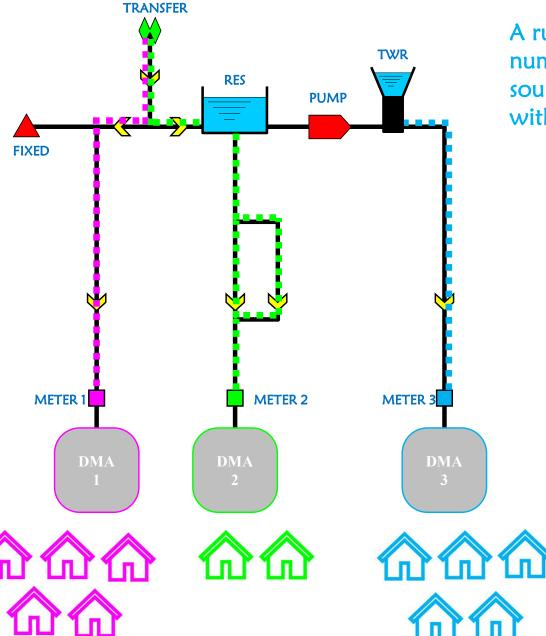
A ruby script is used to count the number of customers supplied via the source, asset, trunk main and meter within the HDZ.
